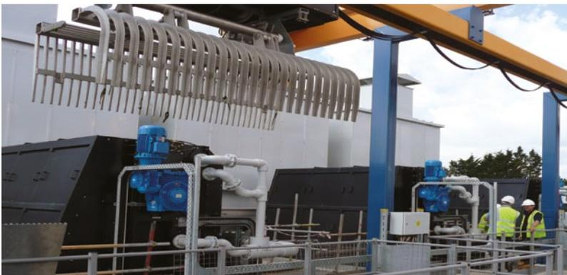
The robust design of the Brackett Green® Traveling Band Screen is highlighted by the robust headshaft construction of these screens awaiting dispatch.
