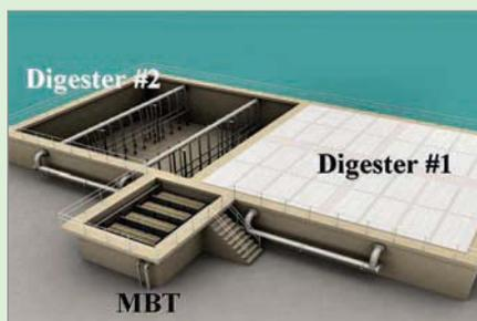
FIGURE 2: Dundee, MI - Typical PAD-K MBR Thickener/Digestion Process Layout
