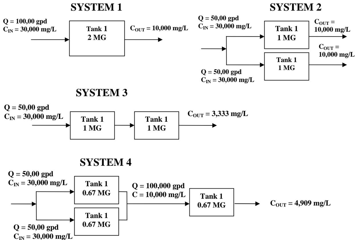
**Table 2: Total Solids Removal of Various CFSTR System Configurations**
