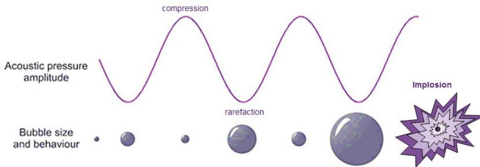
**Figure 1 - Acoustic Cavitation**
