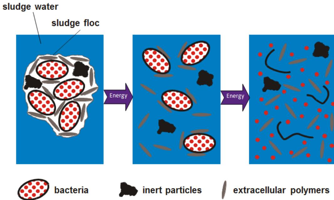
**Figure 4 - Ultrasonic Sludge Disintegration**
