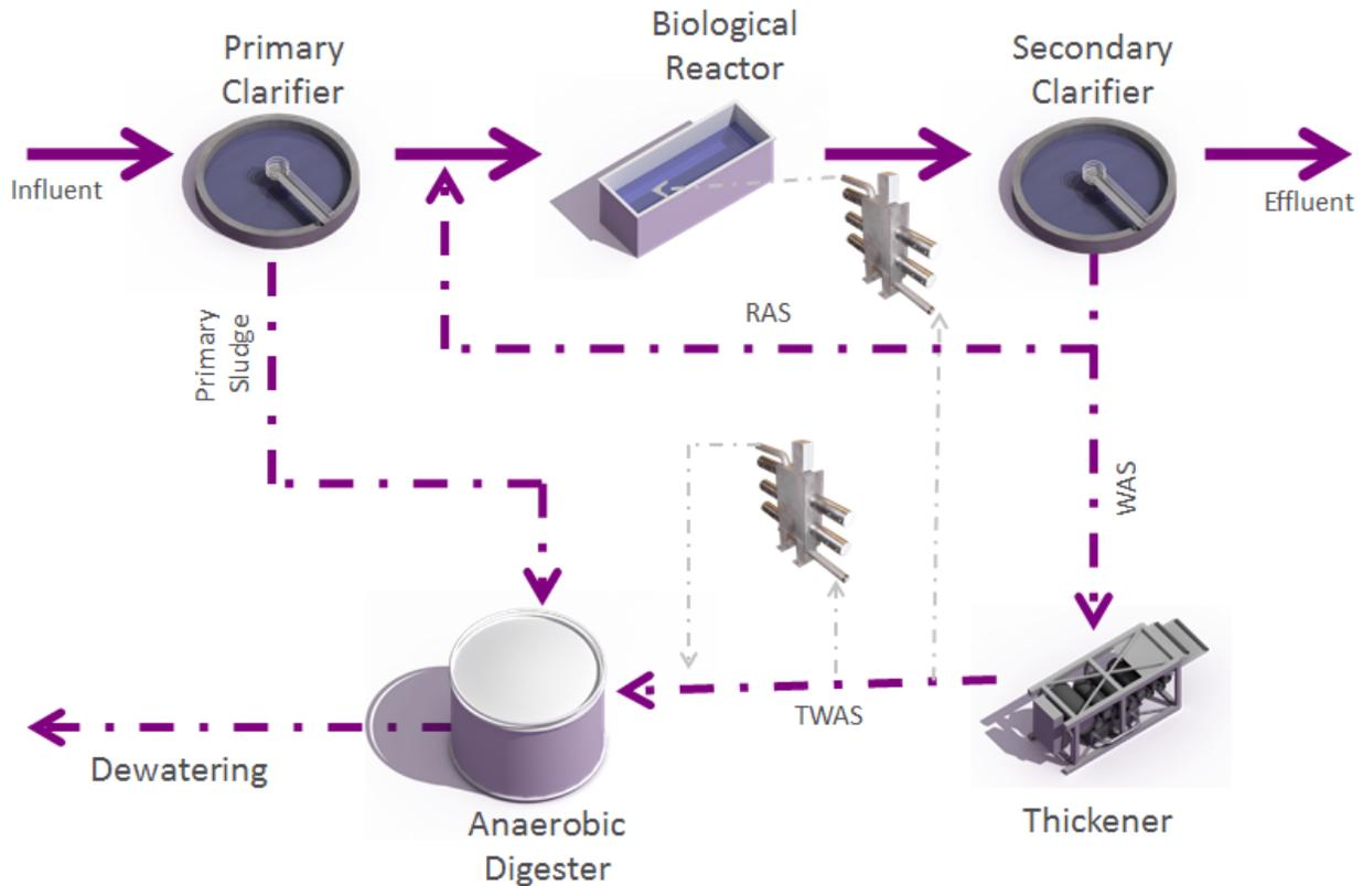
**Figure 3 - Ultrasonic Reactor Placement Locations**
